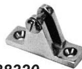
#88320 90° Deck Hinge 7/8" x 2" base, 1/4 - 20 panhead screw included. Drilled for #10 screws.
