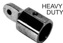
#88396 Outside Eye End for 7/8" tube. Uses 1/4" bolt.
